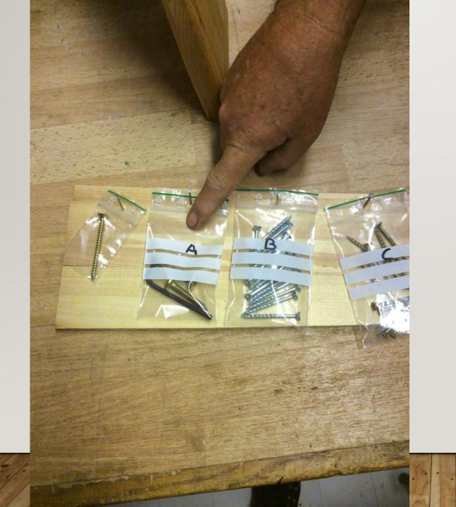
Next step is to put these parts together, use screw A x2 in the two biggger holes.
